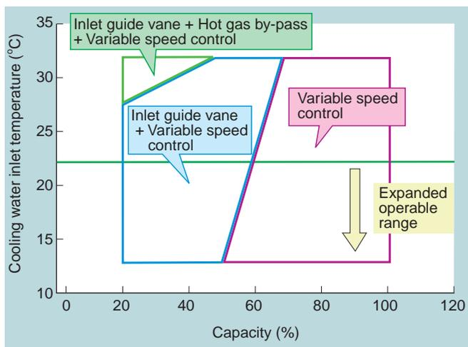
Fig. 7 Schematic diagram for operation range and control system
