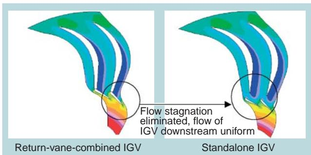
**Fig. 4 Examination of two-stage IGV location based on flow analysis**
