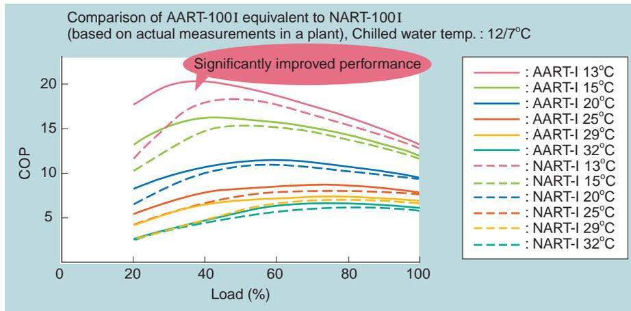
Fig. 9 Comparison of estimated COP for previous model (NART-I) and new model (AART-I) (variable-speed models)
