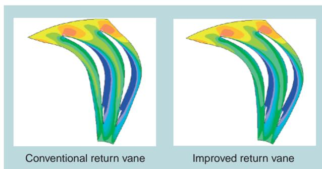
**Fig. 5 Return vane improved based on flow analysis**
