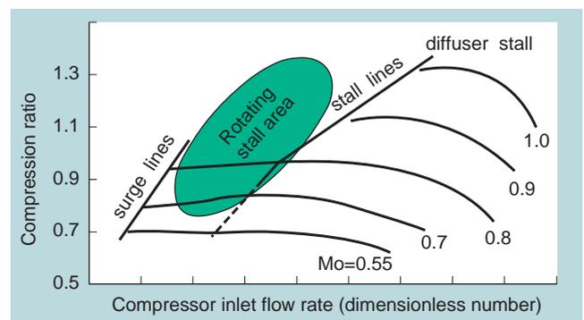
**Fig. 6 Map of Aerodynamic Properties to Illustrate the Improvements**
