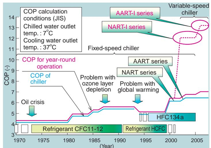
Fig. 1 Trends in turbo chiller performance and refrigerant
