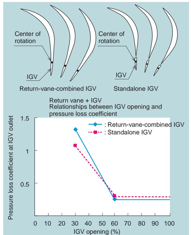
**Fig. 3 Comparison of two-stage IGV location and pressure loss in compressor**
