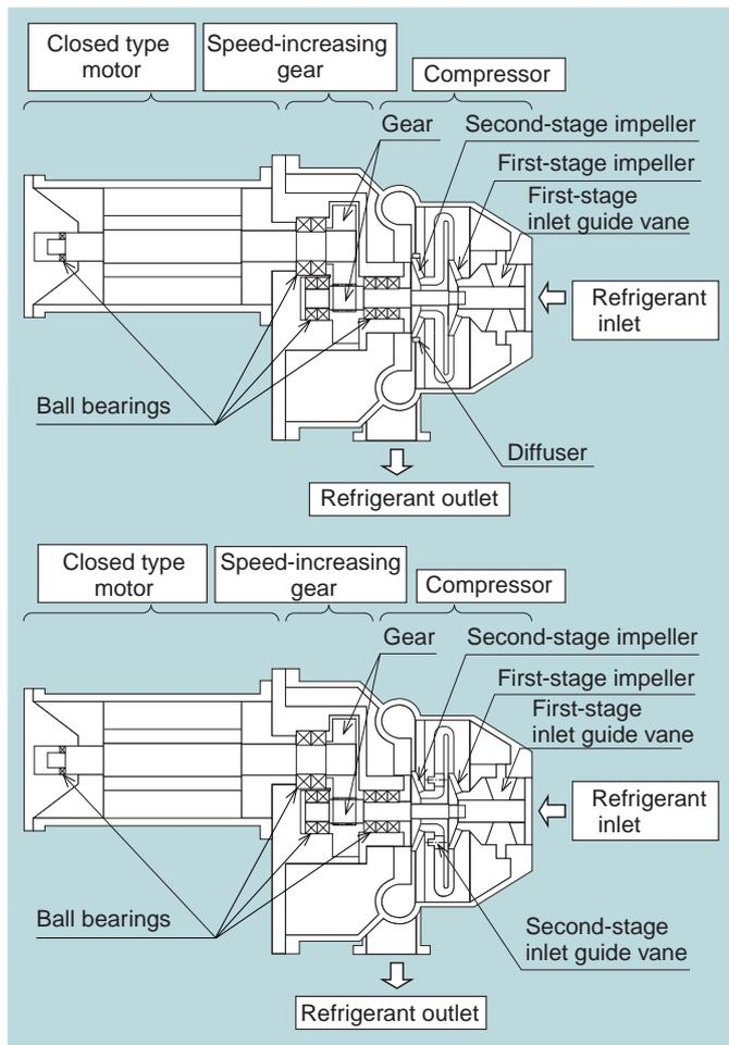
**Fig. 2 Structure of second-stage inlet vane**
